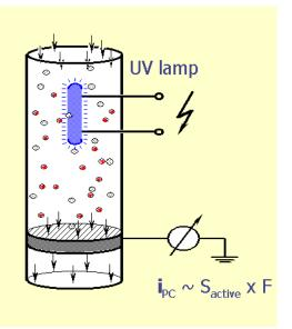
I<sub>PAS</sub> = PAS Current S<sub>active</sub> = Particle active surface area F = Surface chemistry factor
